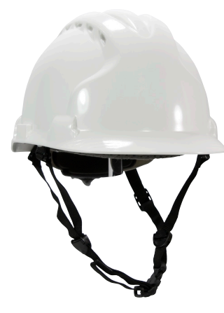
MK8 Evolution® Type II Linesman Hard Hat with HDPE Shell, EPS Impact Liner, Polyester Suspension, Wheel Ratchet Adjustment and 4-Point Chin Strap 280-AHS240
