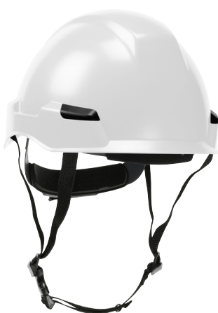
Rocky™ Industrial Climbing Helmet with Polycarbonate / ABS Shell, Hi-Density Foam Impact Liner, Nylon Suspension, Wheel Ratchet Adjustment and 4-Point Chin Strap 280-HP142R
